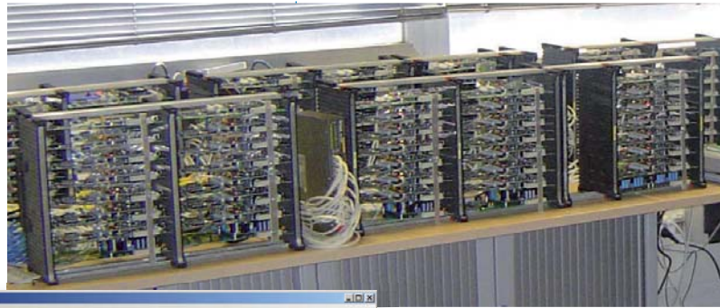
Testbed for heavy traffic conditions based on a special rack with more than one hundred CPU boards equipped with Ethernet cards and connected through switches
